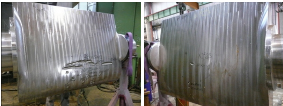
Fig. 4. Francis wicket blades: Excavation and welding repair of casting defects
