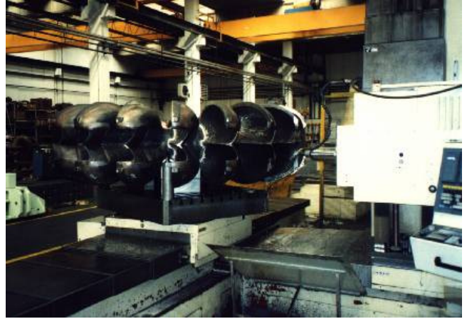
Fig. 4 – CNC milling of bucket's profile
