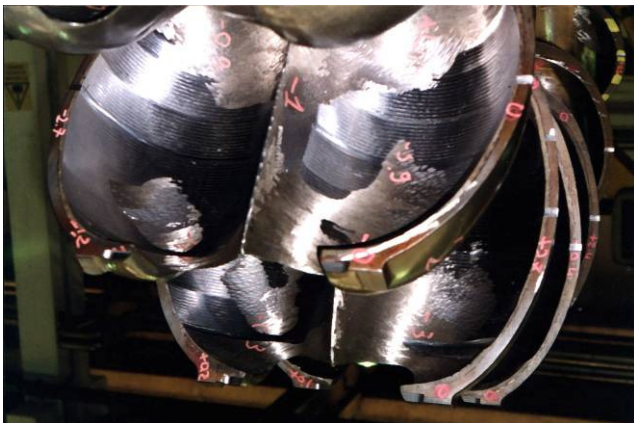
Fig. 3 – Preliminary CNC machining – also shown are the “spots” in the milled surface
