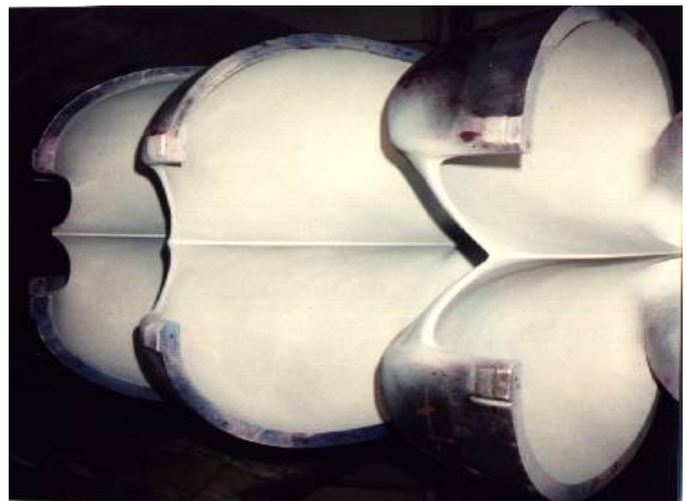
Fig. 5 – Non-destructive inspection (PT)
