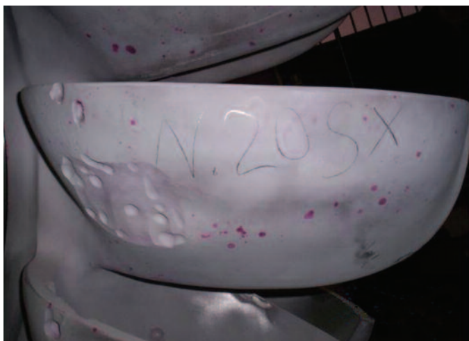
Figure 2. Example of defects on a Pelton runner and white metal bearing segments detected during a liquid penetrant examination.
