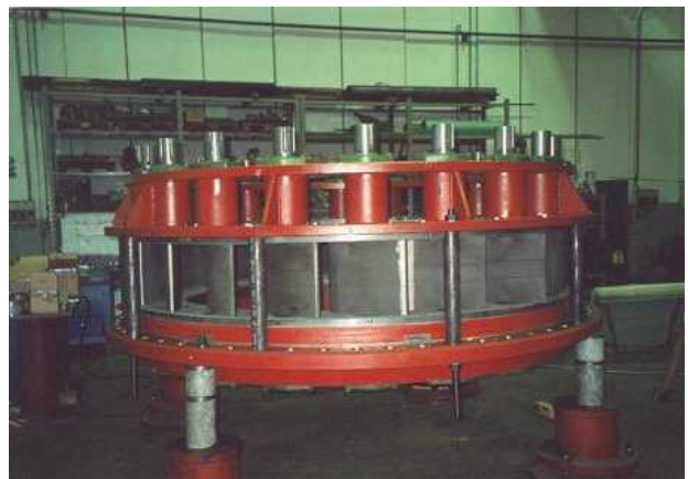
Fig. 4 – pre-assembly in FRAVIT workshop (simulation of the actual conditions on site).
