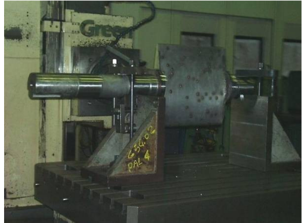
Fig. 3 – repairing of guide blades
