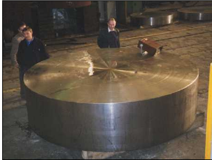
Fig. 5. Forged disk for a new Pelton runner
