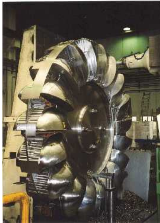
Fig. 2. CNC-Machining of a Pelton runner made from a forged disk at FRAVIT's
