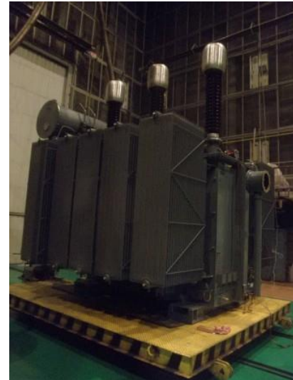
Transformer during the FAT tests
