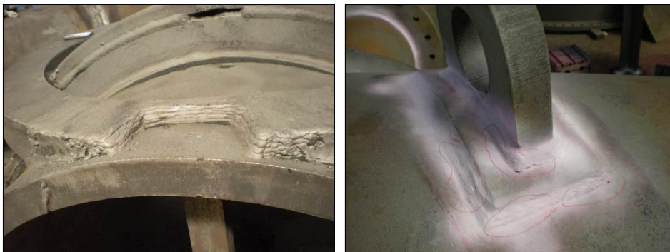
Figure 3. Example of welding defects
