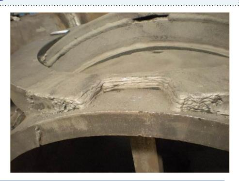
Example of POOR WELD PREPARATION AND OF POOR QUALITY WELD ON A ROTARY VALVE
