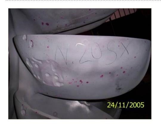
Example of excavation of DEFECTS ON A CAST PELTON RUNNER
