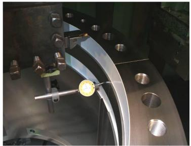
Dimensional check of TURBINE SHAFTS AND COVERS against construction drawings
