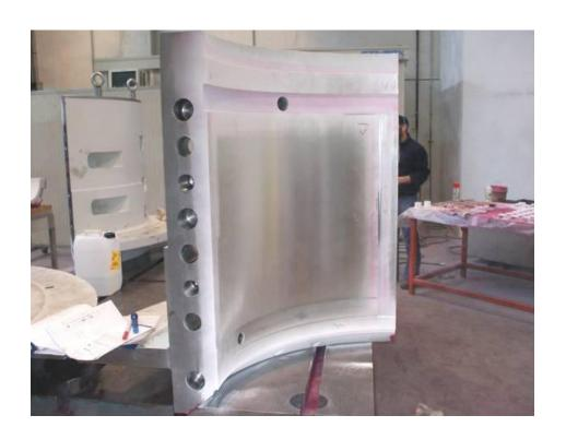
Non-destructive examination by LIQUID PENETRANT on a WHITE METAL BEARING
